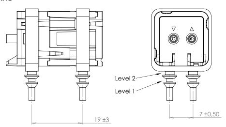
Level 1: Drill hole 4 x Ø3 mm Level 2: Drill hole 4 x Ø3,5 mm
