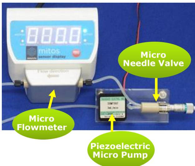
The Low Pulsation Micro Pump Module is a module to adjust the flow of a piezoelectric micro pump at the  $\mu\text{l}/\text{min}$  level using a micro needle valve. In the setup in the left picture, the output flow from the module is being measured by a micro flowmeter. The features of this module make it suitable for various fields, such as flow cytometers, cell culture equipment, etc.
